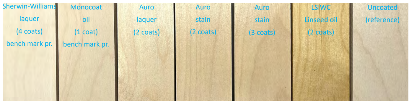
Results of different coatings on the same type of wood
