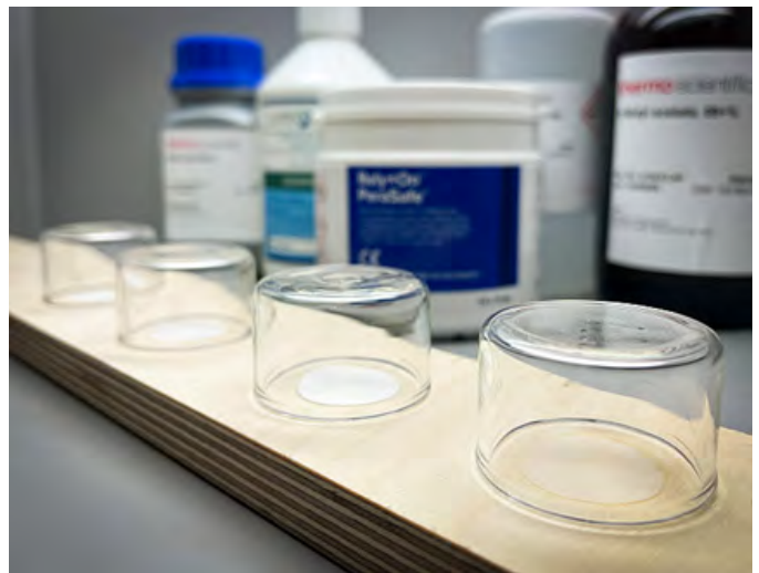
Testing of chemical resistance of coatings to different liquids
